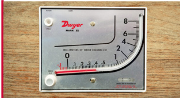
Figure 99 A manometer used to monitor air pressure within the house (the reading given is equivalent to 0.15 inches of water column).
