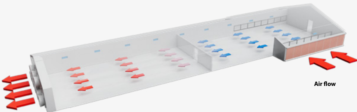
Figure 108 Air flow in a tunnel ventilated house.
