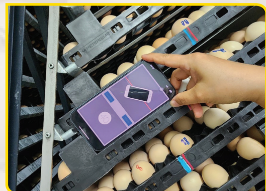
Measuring turning angles using an app such as Angle Meter Pro.
