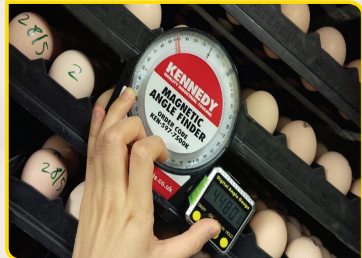
Measuring turning angle with a dial and a digital meter.
